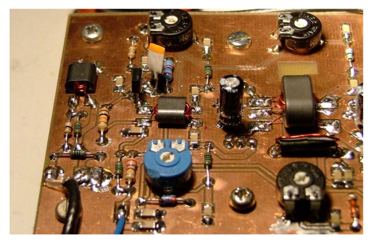
Picture showing component mounting methods and a melted preset.. it was the prototype!
