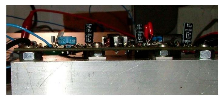
Method I used to space PCB from heatsink, note the carefully chosen nuts and washers used as spacers.
