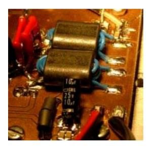
Output transformer mounting detail.
