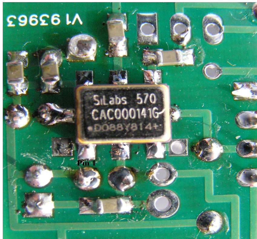
Fig 4 Location of S570 chip – Bottom left pin is Pin 1 aligned with dot on Si571
